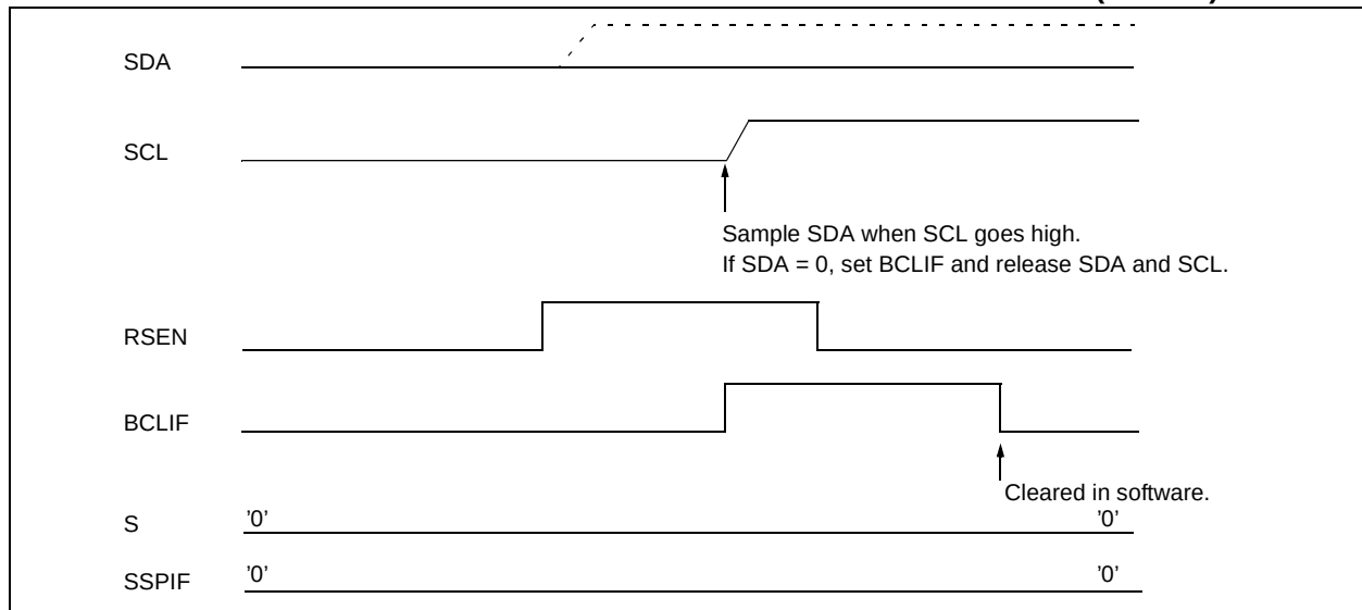
FIGURE 15-38: BUS COLLISION DURING A REPEATED START CONDITION (CASE 1)
