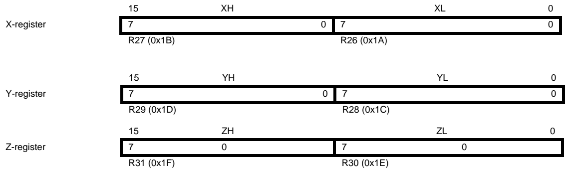
Figure 5-3. The X-, Y-, and Z-registers
