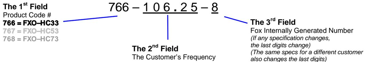
**This example, FXO-HC335R-106.25 = HCMOS Output, Ceramic 3.2 x 2.5mm Package, 3.3V, ±50 PPM Stability, -40 to +85°C Temperature Range, at 106.25 MHz**
