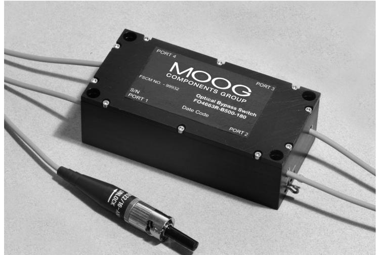
The multimode 2x2 moving-mirror optical bypass switch meets all the requirements of the FDDI Physical Medium Dependent (PMD) standard and SAFENET specifications for fiber optic data network applications. The highly reliable performance of the device is made possible by its unique silicon micromachine based switch design. A sealed, ruggedized housing isolates the optical components from external shock and vibration effects.
