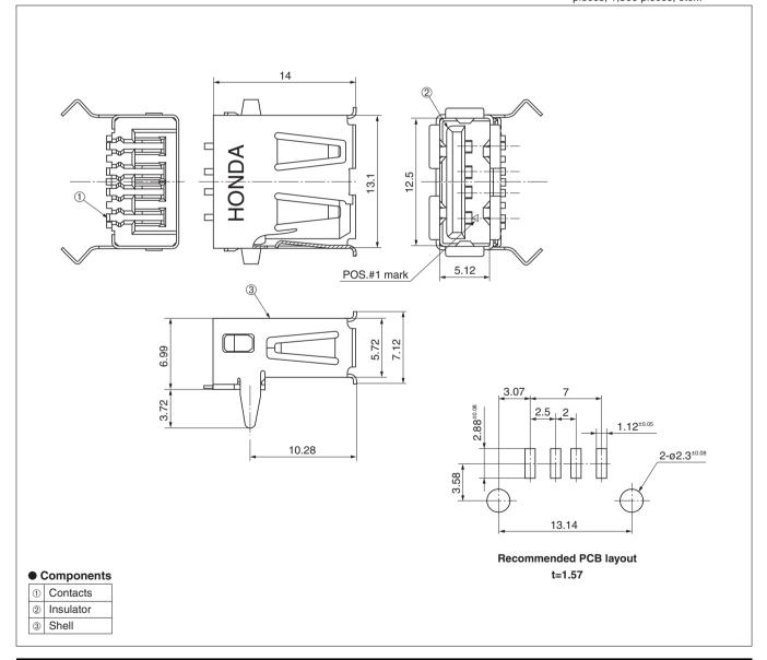
Mating connectors: USB A series connector for cable (USB 2.0 standard)
