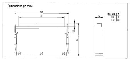
BKS-S39-D32 for use with BALLUFF BTA-P (Digital Card used with BTL-P Transducer)
