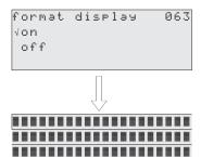
With this function, you activate a test for the LC display. All points on the display are activated for around 2 seconds.
