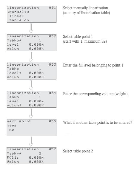
Continue either until 32 table points have been selected or until manual entry of the linearization table is completed by selecting "next point = no".
