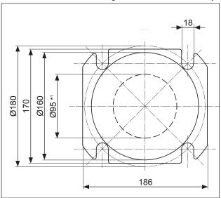
\*1 Minimum dimension for installing the wiper mechanism and standard weight
