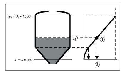
Each point ① in the linearization table is described by a pair of values: ② fill level and volume (or weight) ③.
