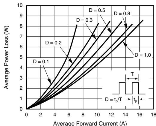
Fig. 2 - Forward Power Dissipation Characteristics Per Diode
