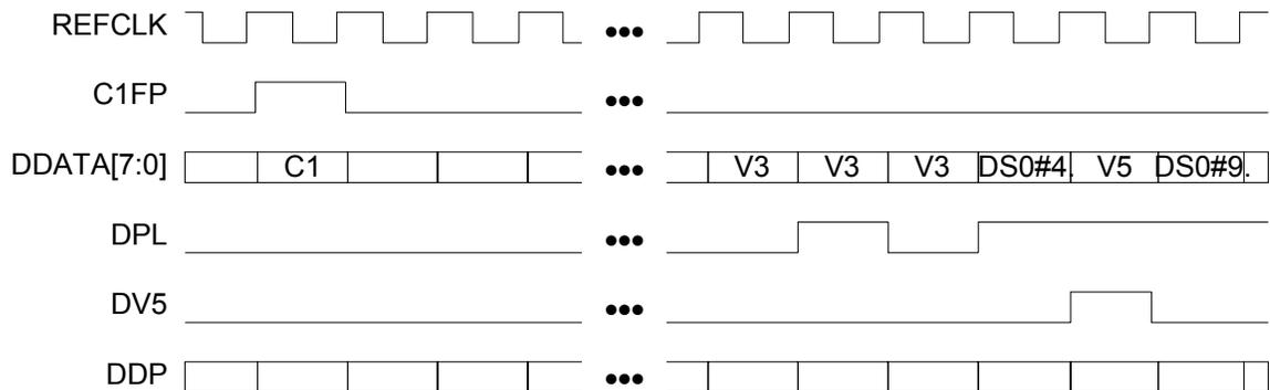
Figure 11 illustrates the operation of the SBI DROP BUS, using a negative justification on the second to last V3 octet as an example. The justification is indicated by asserting DPL high during the V3 octet. The timing diagram also shows the location of one of the tributaries by asserting DV5 high during the V5 octet.
