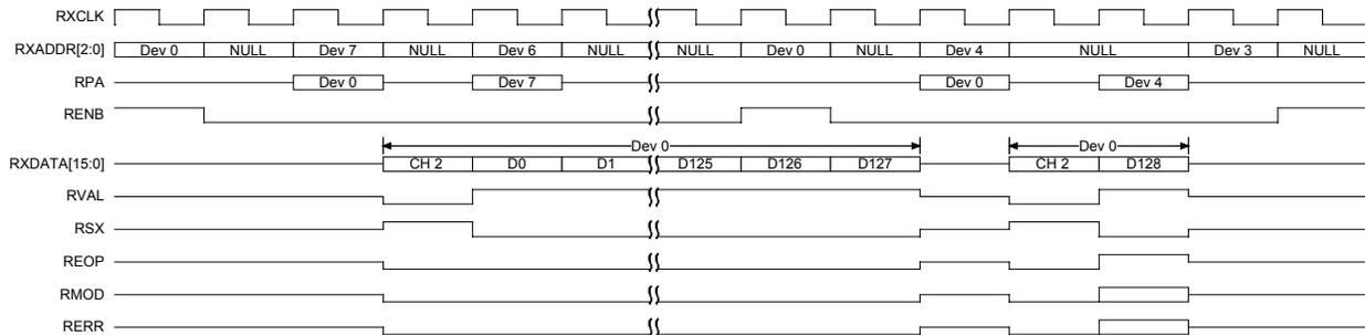
Figure 18 shows optimal bandwidth utilization across the Rx APPI.
