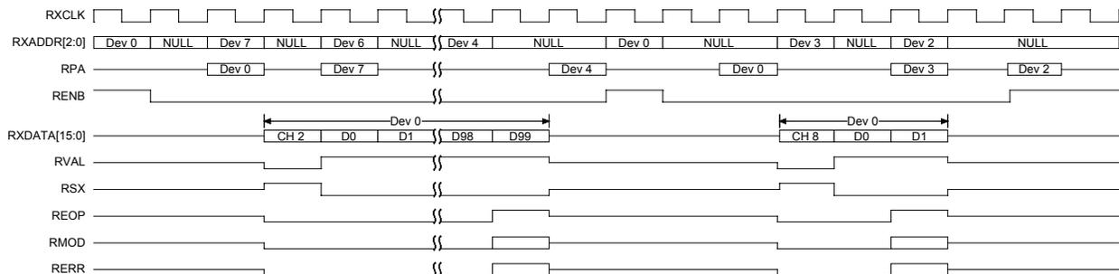
Figure 17 shows the transfer of a 100 word packet across the Rx APPI from FREEDM-84A672 device 0, channel 2 followed by the transfer of a 2 word packet from FREEDM-84A672 device 0, channel 8. More importantly, Figure 17 illustrates that, for back-to-back transfers from the same FREEDM-84A672
