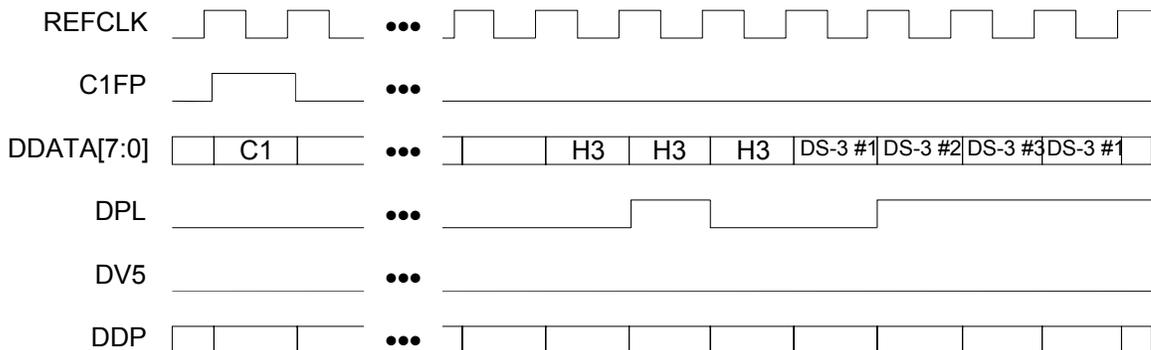
Figure 12 shows three DS-3 tributaries mapped onto the SBI bus. A negative justification is shown for DS-3 #2 during the H3 octet with DPL asserted high. A positive justification is shown for DS-3#1 during the first DS-3#1 octet after H3 which has DPL asserted low.
