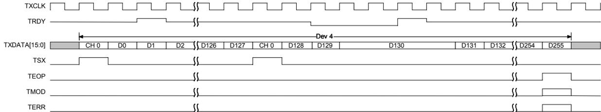
Figure 20 shows transfer of a 256 word packet on the Tx APPI of FREEDM-84A672 device 4, channel 0. The maximum burst data transfer (excluding channel address prepend) is 128 words, so two data transfers are required to complete the transfer of the 256 word packet.
