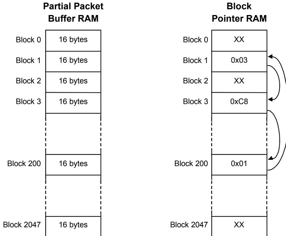
The partial packet buffer processor is divided into three sections: reader, writer and roamer. The roamer is a time-sliced state machine which tracks each channel's FIFO buffer free space and signals the writer to service a particular channel. The writer requests data from the TAPI672 block and transfers packet data from the TAPI672 to the associated channel FIFO. The reader is a time-
