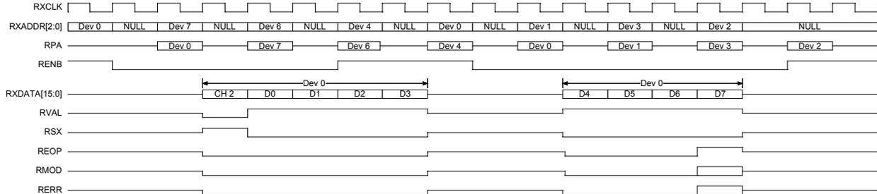
Figure 16 shows the transfer of an 8 word packet across the Rx APPI from FREEDM-84A672 device 0, channel 2. In this example, seven FREEDM-84A672 devices are sharing the Rx APPI, with device 5 being the null address.
