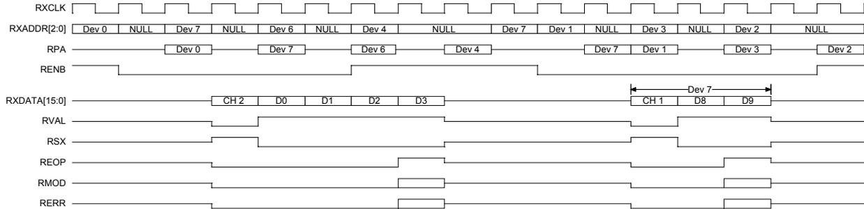
Figure 19 shows the boundary condition where a packet transfer completes shortly after the external controller has set RENB high to pause the FREEDM-84A672 device. The second data transfer is the final two words of a packet for FREEDM-84A672 device 7, channel 1.
