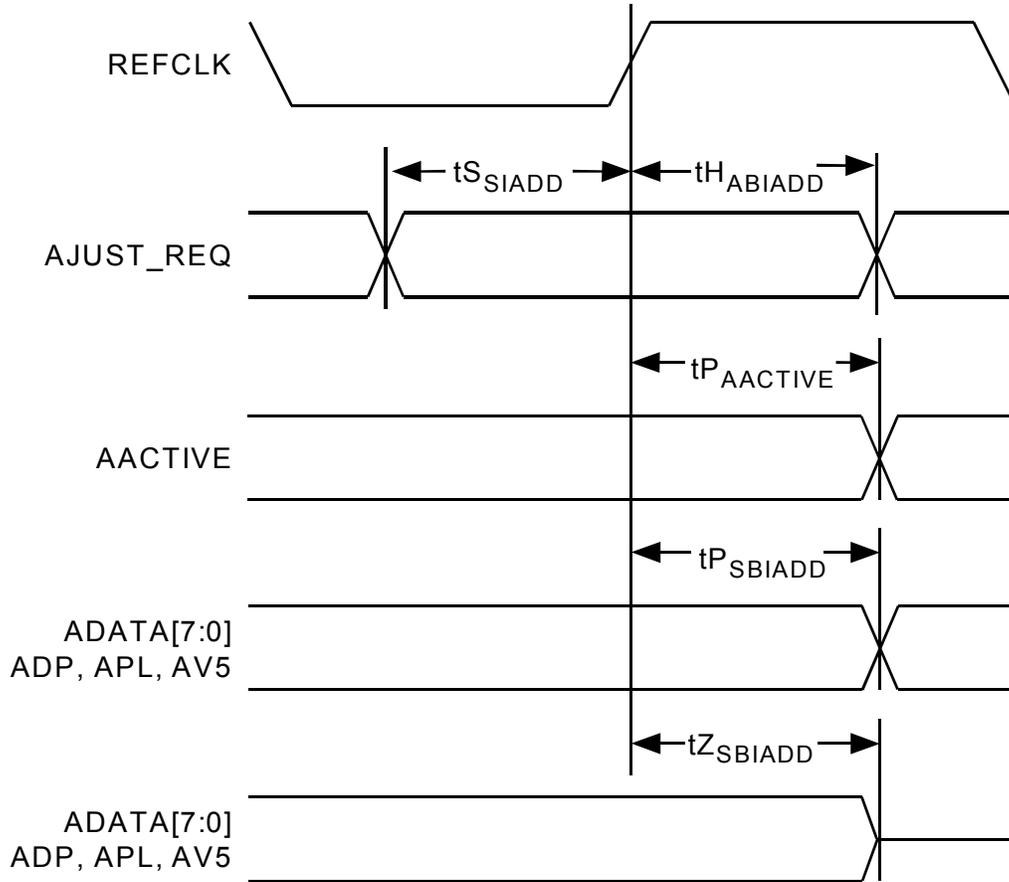
**Figure 26 – SBI ADD BUS Collision Avoidance Timing**
