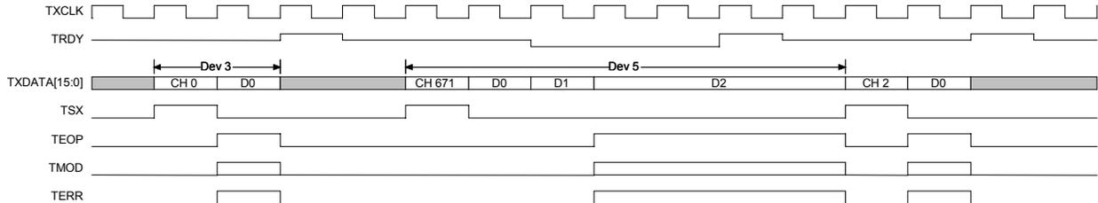
Figure 21 shows two special conditions – (1) the transfer of a one word packet illustrating how the external controller must wait until TRDY has been sampled high before the next data transfer can begin, and (2) the transfer of a packet which completes when TRDY is set low illustrating that although the packet has been completely transferred, the external controller must still wait until TRDY has been sampled high before the next data transfer can begin.
