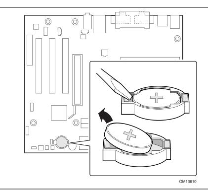
Figure 14. Removing the Battery
