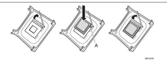
Figure 6. Installing a Processor
