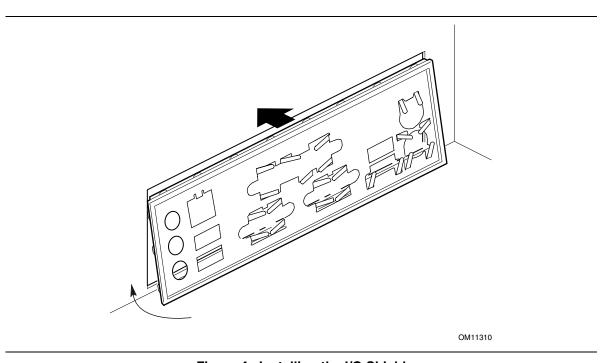
Figure 4. Installing the I/O Shield
