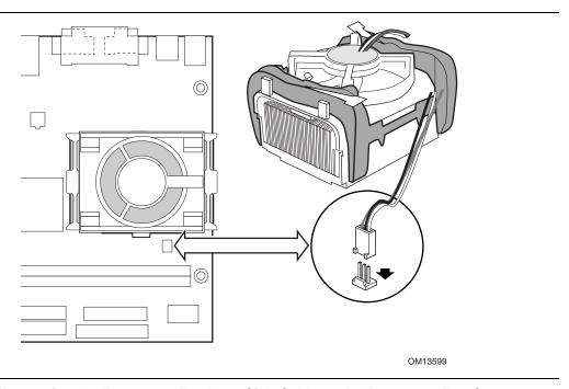
Figure 7. Connecting the Processor Fan Heat Sink Cable to the Processor Fan Connector
