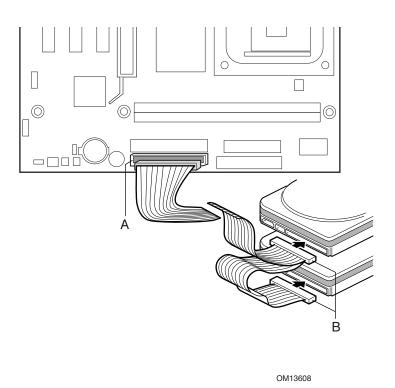
Figure 10. Connecting the IDE Cable
