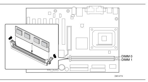
Figure 8. Installing a Memory Module
