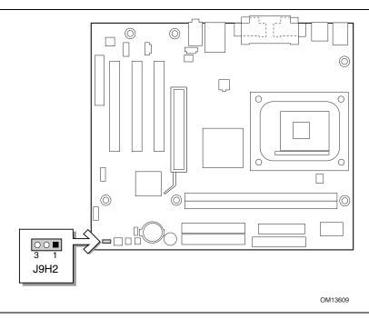
Figure 13. Location of the BIOS Configuration Jumper Block
