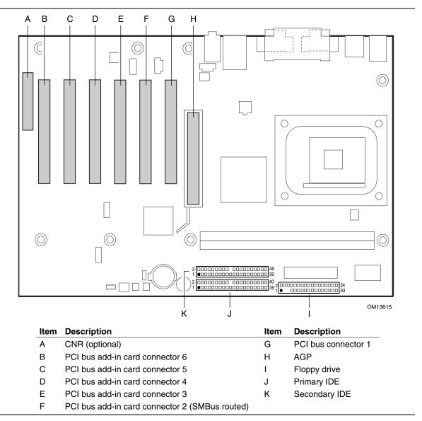
Figure 17. PCI Bus Add-in Card and Peripheral Interface Connectors
