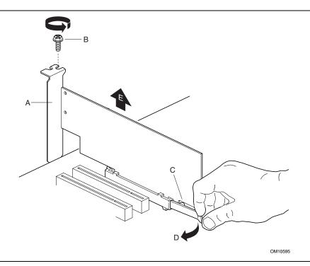
Figure 9. Removing the AGP or ADD Card
