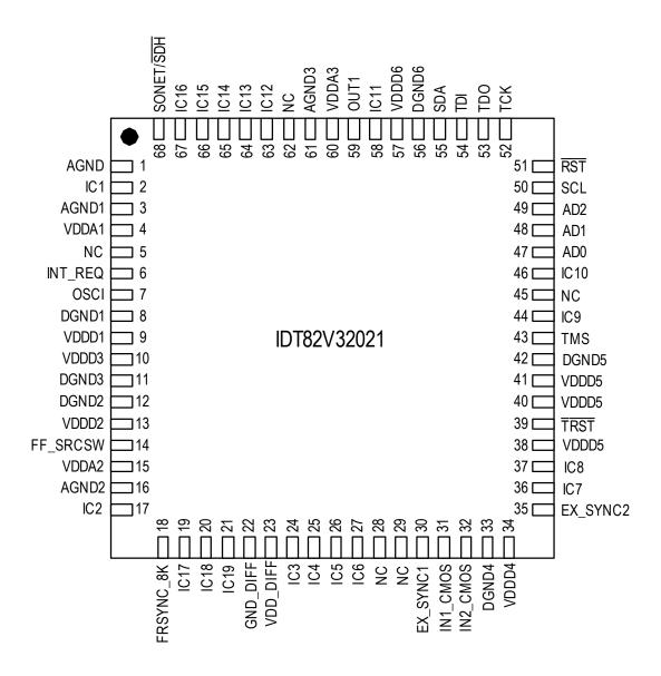
Figure 2. Pin Assignment (Top View)
