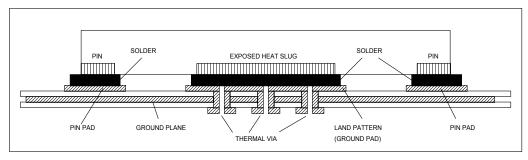
Figure 18. Assembly for Expose Pad thermal Release Path (Side View)
