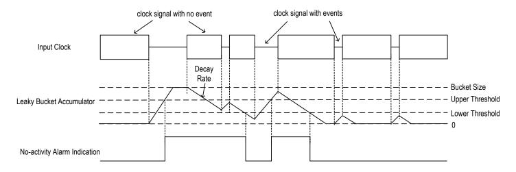
Figure 4. Input Clock Activity Monitoring
