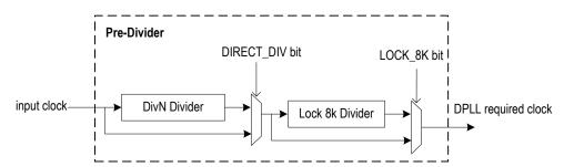
Figure 3. Pre-Divider for An Input Clock
