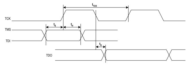
Figure 17. JTAG Interface Timing Diagram
