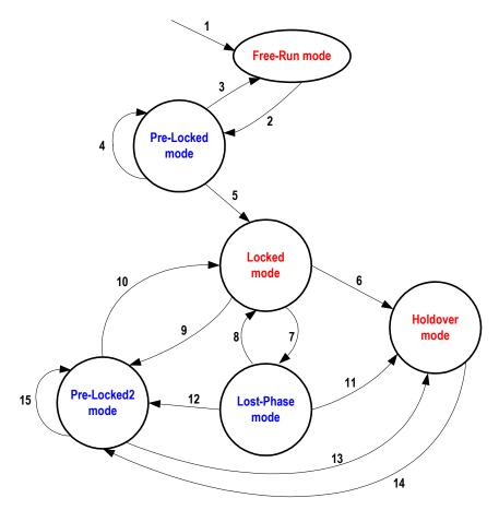
Figure 6. T0 Selected Input Clock vs. DPLL Automatic Operating Mode
