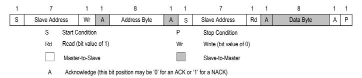
Figure 14. Slave-transmitter Mode
