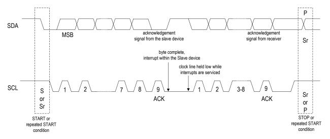
Figure 12. Data Transfer on the I<sup>2</sup>C-bus
