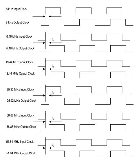
Figure 20. Input / Output Clock Timing
