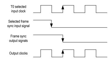
Figure 8. 0.5 UI Early Frame Sync Input Signal Timing
