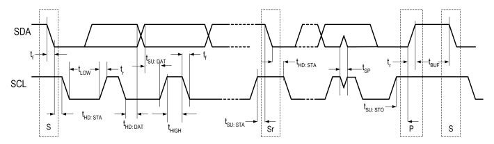
Figure 16. Timing Definition of I<sup>2</sup>C-bus
