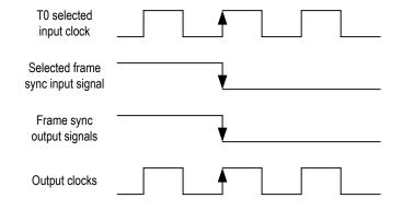
Figure 7. On Target Frame Sync Input Signal Timing
