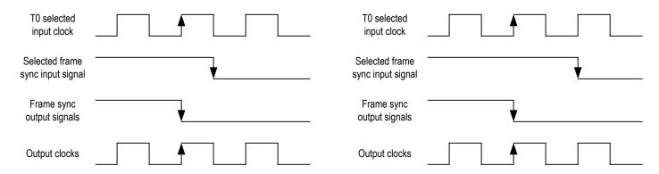
Figure 9. 0.5 UI Late Frame Sync Input Signal Timing
