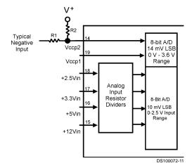
FIGURE 6. Input Examples. Resistor values shown in table provide approximately 1.25V at the Vccp inputs.
