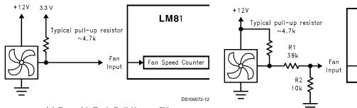
(a) Fan with Tach Pull-Up to +5V
