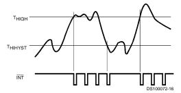
\*Note: Interrupt resets occur only when interrupt Status Register 1 is read.
