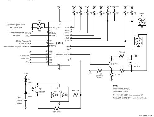
FIGURE 19. In this PC application the LM81 monitors temperature, fan speed for 2 fans, and 6 power supply voltages. It also monitors an optical chassis intrusion detector.
