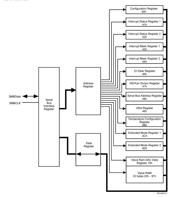
FIGURE 4. LM81 Register Structure
