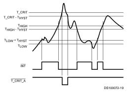
\*Note: Interrupt resets occur only when interrupt Status Register 1 is read.
