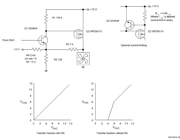
FIGURE 8. Amplifier circuit for connection between DAC output and fan.
