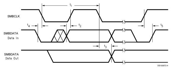
FIGURE 1. Serial Bus Timing Diagram
