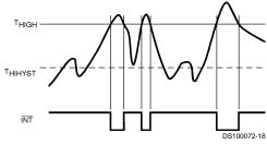
\*Note: Interrupt resets occur only when interrupt Status Register 1 is read.
