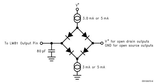
FIGURE 3. Digital Output Load Test Circuitry
