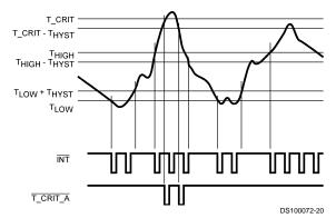
\*Note: Interrupt resets occur only when interrupt Status Register 1 is read.
