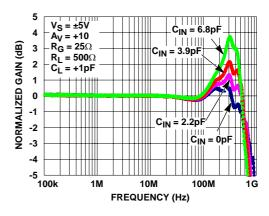
FIGURE 14. GAIN vs FREQUENCY FOR VARIOUS  $C_{IN}(-)$  ( $A_V = +10$ )
