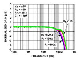
FIGURE 9. GAIN vs FREQUENCY FOR VARIOUS  $R_{LOAD}$  (A<sub>V</sub> = +20)
