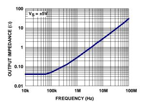
FIGURE 17. OUTPUT IMPEDANCE vs FREQUENCY
