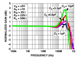
FIGURE 10. GAIN vs FREQUENCY FOR VARIOUS  $C_{LOAD}$  ( $A_V = +10$ )
