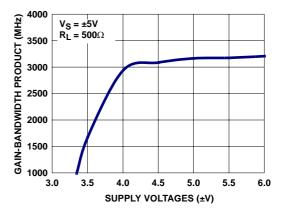
FIGURE 6. GAIN BANDWIDTH PRODUCT vs SUPPLY VOLTAGES
