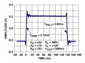
FIGURE 29. SMALL SIGNAL STEP RESPONSE\_RISE AND FALL TIME
