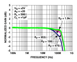
FIGURE 13. GAIN vs FREQUENCY FOR VARIOUS  $R_F$  ( $A_V = +20$ )
