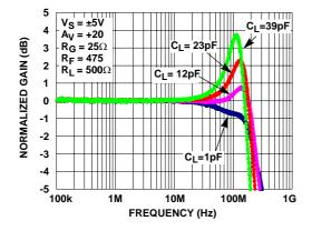
FIGURE 11. GAIN vs FREQUENCY FOR VARIOUS  $C_{LOAD}$  ( $A_V = +20$ )
