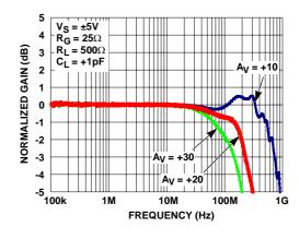
FIGURE 4. GAIN vs FREQUENCY FOR VARIOUS +AV
