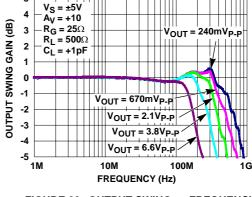
FIGURE 20. OUTPUT SWING vs FREQUENCY
