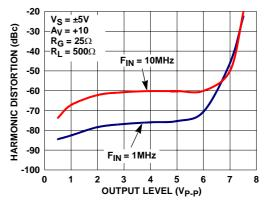
FIGURE 24. TOTAL HARMONIC DISTORTION vs OUTPUT VOLTAGE
