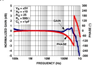
FIGURE 1. GAIN & PHASE vs FREQUENCY
