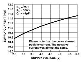
FIGURE 31. SUPPLY CURRENT vs SUPPLY VOLTAGE
