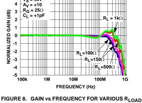
FIGURE 8. GAIN VS FREQUENCY FOR VARIOUS R<sub>LOAD</sub>  $(A_V = +10)$
