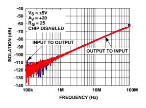
FIGURE 22. INPUT AND OUTPUT ISOLATION
