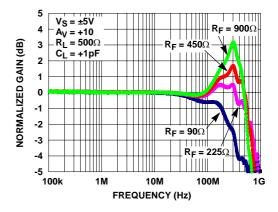
FIGURE 12. GAIN vs FREQUENCY FOR VARIOUS  $R_F$  ( $A_V = +10$ )
