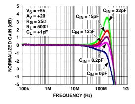
FIGURE 15. GAIN vs FREQUENCY FOR VARIOUS  $C_{IN}$  ( $A_V = +20$ )
