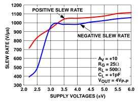
FIGURE 32. SLEW RATE vs SUPPLY VOLTAGES
