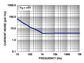
FIGURE 28. EQUIVALENT INPUT CURRENT NOISE vs FREQUENCY
