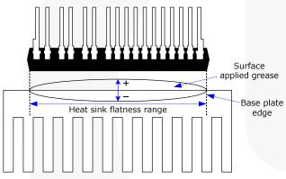
Figure 3. Measurement Point of Heat Sink Flatness
