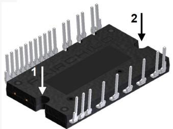
Figure 1. Mounting Screws Fastening Order: Pre-Screwing:  $1 \rightarrow 2$ ; Final Screwing:  $2 \rightarrow 1$
