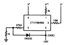
$V^+$  = +20V FOR LT107XM, +40V FOR LT107XHVM  $V^{++}$  = +45V FOR LT107XM, +55V FOR LT107XHVM X = 0, 1, OR 2
