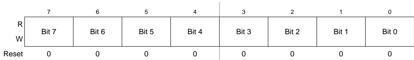
Figure 8-4. CRC High Register (CRCH)
