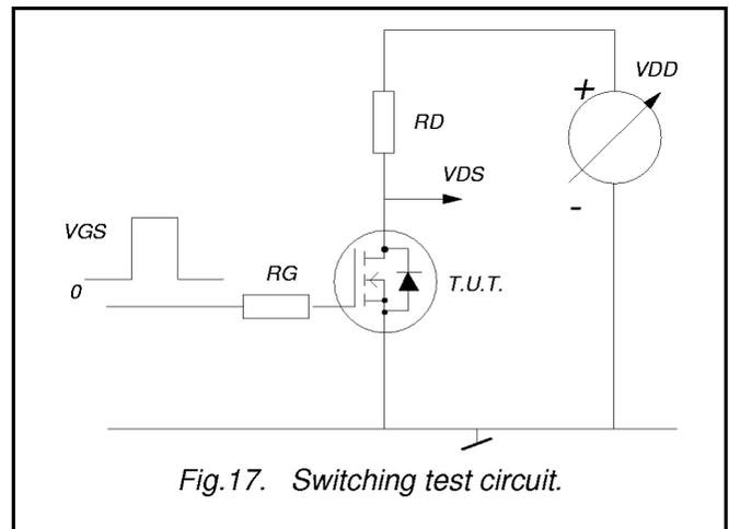
Fig.17. Switching test circuit.
