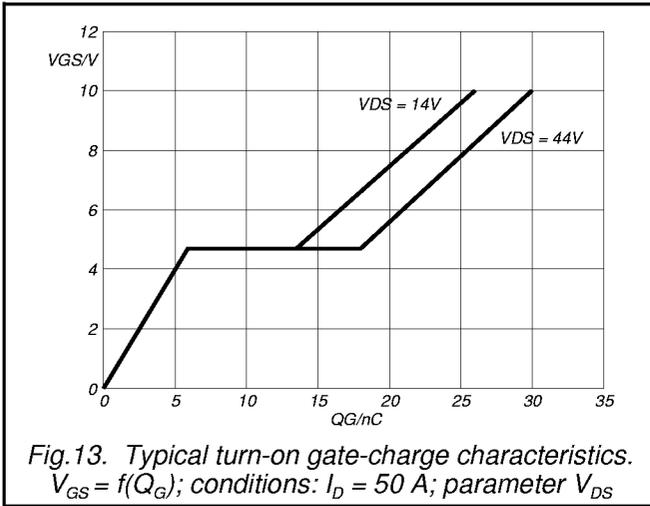
Fig.13. Typical turn-on gate-charge characteristics.
