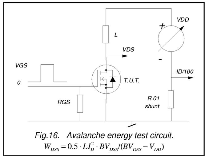
Fig.16. Avalanche energy test circuit.
