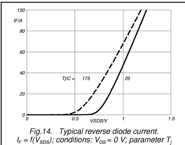
Fig.14. Typical reverse diode current.
