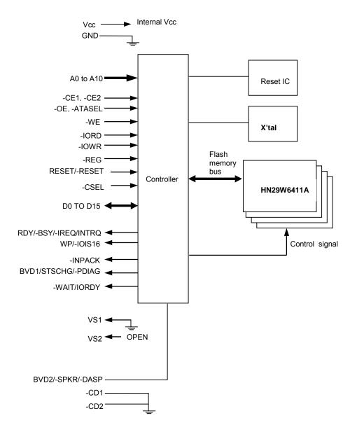
Note: -CE1, -CE2, -OE, -WE, -IORD, -IOWR, -REG, RESET, -CSEL pins are pulled up in the card. -PDIAG PIN IS Schmitt trigger type input output buffer.
