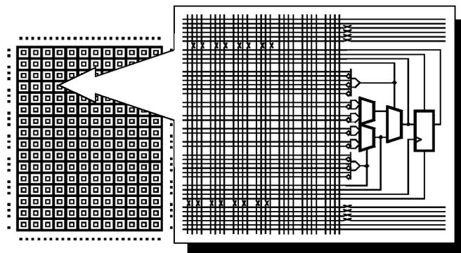
▪ = Up to 80 prog. I/O cells, 6 Input high-drive cells, 2 Input/Clk (high-drive) cells
