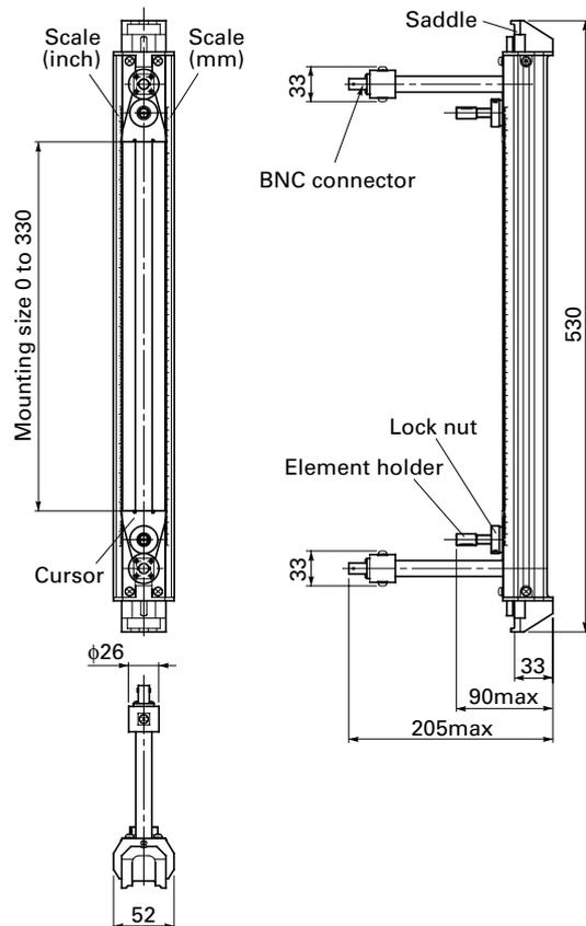
Detector, FLD32 (High-temperature sensor)
