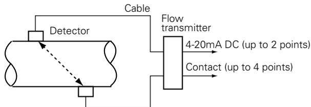
(5) 2-pipe system (with any combination of sensors)
