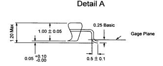
NOTE: All dimensions are in millimeters; Package diagrams are not drawn to scale.
