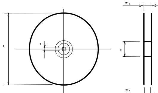
The minimum bending radius is 45 mm.
