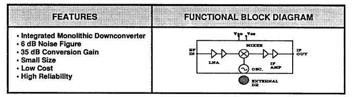
The ANADIGICS Ku-Band MMIC Downconverter is a low-cost, high-volume GaAs MMIC which is suitable for use in the field of consumer electronics.
