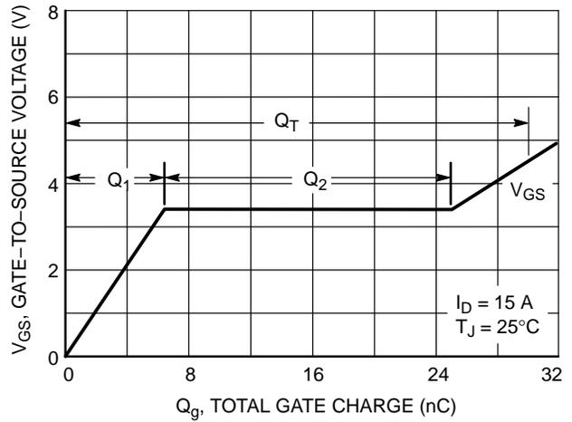
**Figure 8. Gate-to-Source and Drain-to-Source Voltage versus Total Charge**
