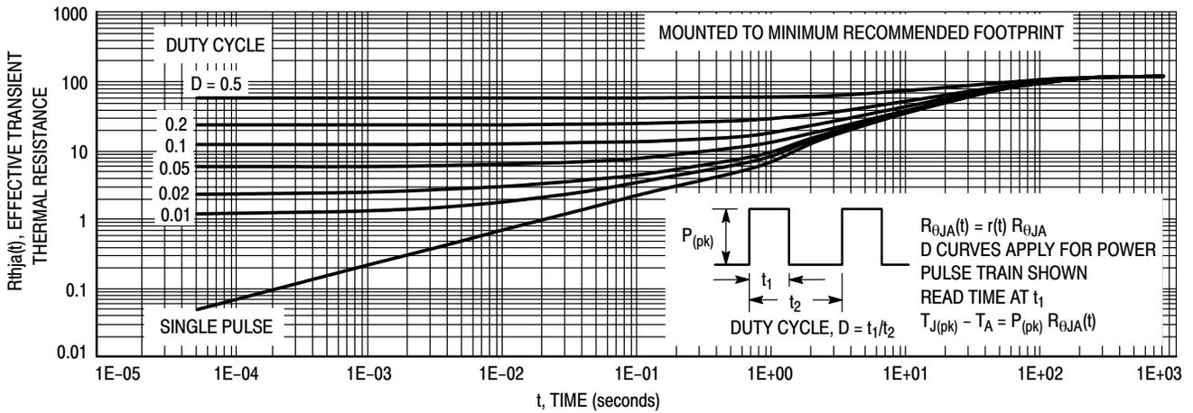
**Figure 13. Thermal Response – Various Duty Cycles**
