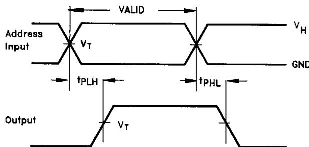
Input and output threshold voltage:
