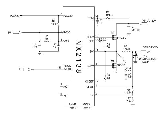
Figure 3 - Demo board schematic
