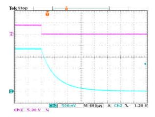
Fig.4 Startup (CH2 1.8V OUTPUT, CH3 PGOOD)
