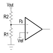
Figure 17 - Voltage Divider
