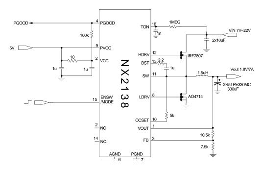
Figure1 - Typical application of NX2138
