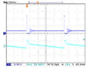
Fig. 9 Output ripple at full load (CH1 SW, CH2 1.8V OUTPUT AC, CH4 OUTPUT CURRENT)
