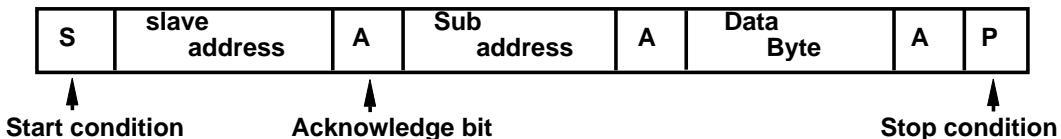
(3) Sub address byte and Data byte format :
