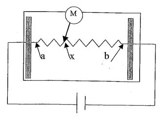
Va: maximum voltage in the active area of touch panel Vb: minimum voltage in the active area of touch panel
