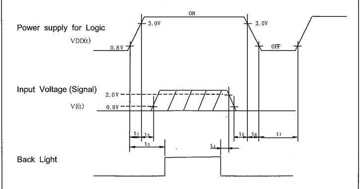
$$\begin{array}{ccc} \underline{\text{POWER ON}} \\ & t_1 \leqq 15\,\text{ms} \\ \\ 0\,\text{ms} < t_2 \leqq 45\,\text{ms} \\ \\ 0. \ 1s \leqq t_3 \end{array}$$
