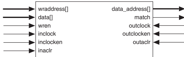
Figure 23. APEX 20KC CAM Block Diagram
