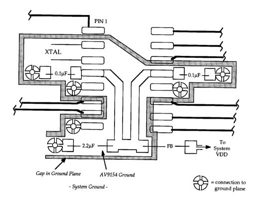
This is the recommended layout for the AV9154 to maximize clock performance. Shown are the power and ground connections, the ground plane, and the input/output traces.
