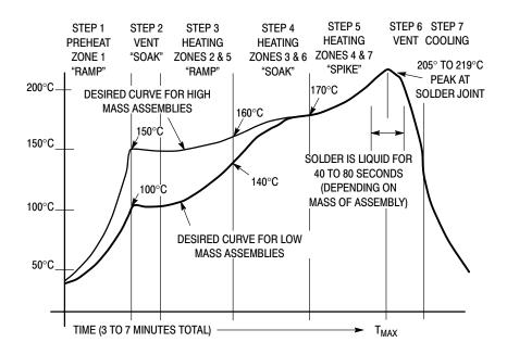
Figure 8. Typical Solder Heating Profile
