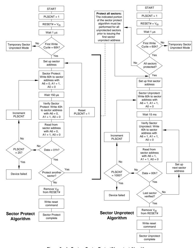
Figure 2. In-System Sector Protect/Unprotect Algorithms
