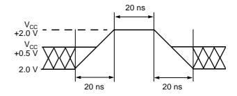
Figure 9. Maximum Positive Overshoot Waveform
