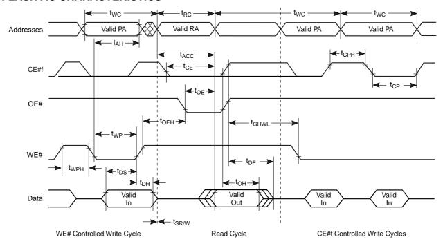
Figure 21. Back-to-back Read/Write Cycle Timings
