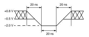
Figure 8. Maximum Negative Overshoot Waveform
