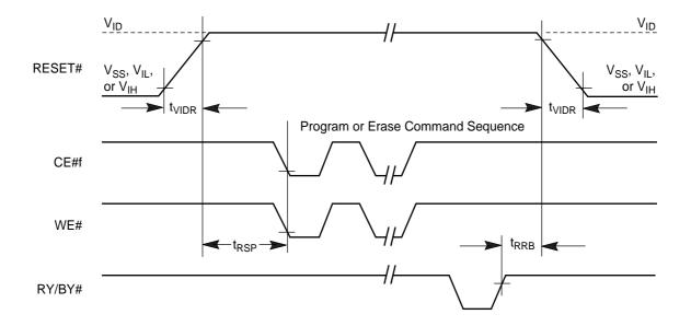
Figure 25. Temporary Sector Unprotect Timing Diagram
