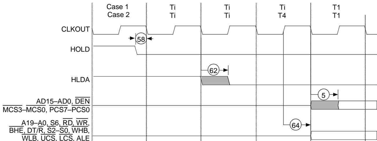
Figure 24. Exiting Bus Hold Waveforms
