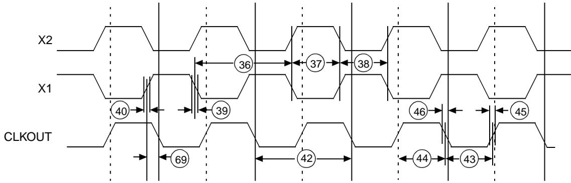
Figure 25. System Clocks Waveforms—Active Mode (PLL 1x Mode)
