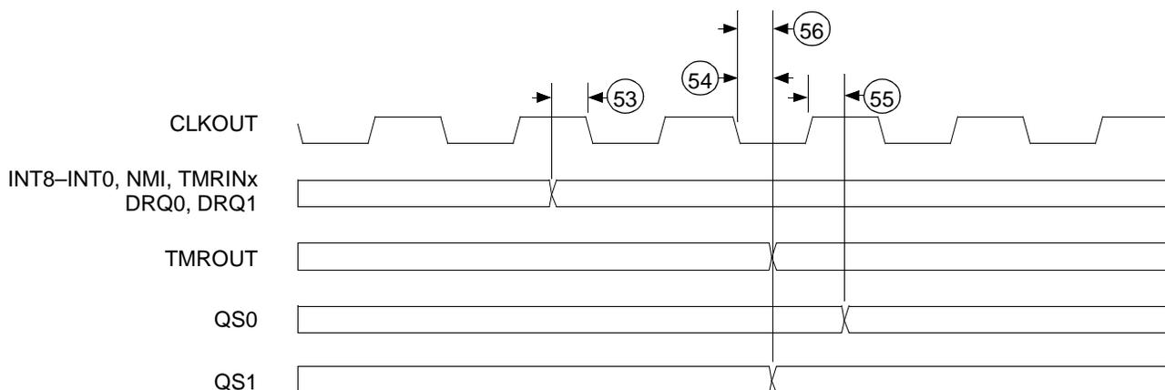
Figure 17. Peripheral Waveforms
