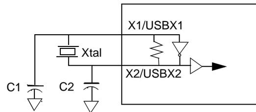
**Figure 7. External Interface to Support Clocks—Fundamental Mode Crystal**
