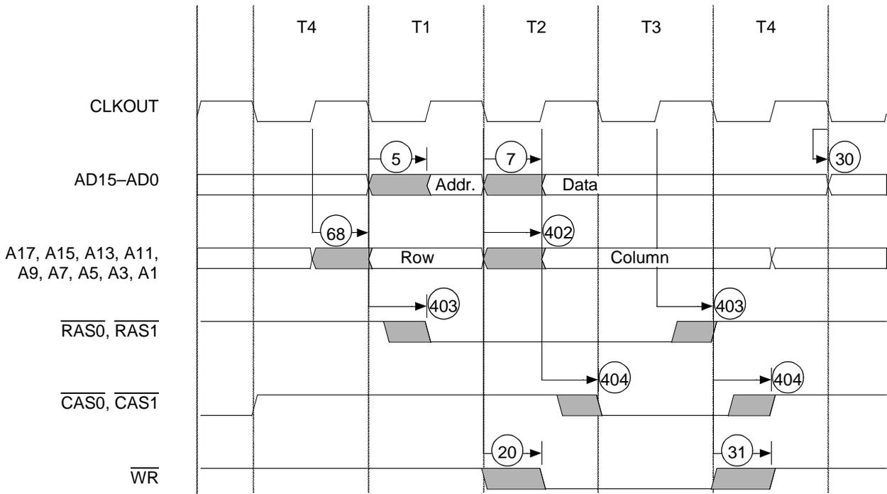
Figure 32. DRAM Write Cycle without Wait States Waveform
