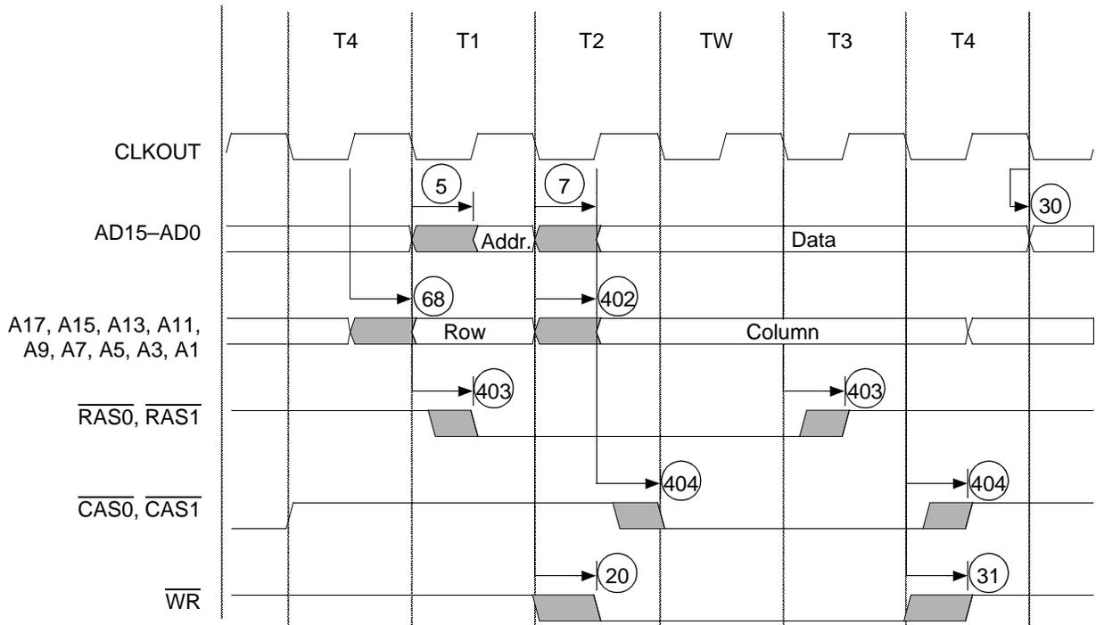
Figure 33. DRAM Write Cycle with Wait States Waveform
