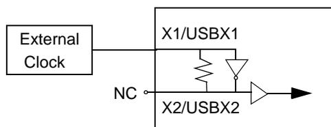
**Figure 8. External Interface to Support Clocks—External Clock Source**
