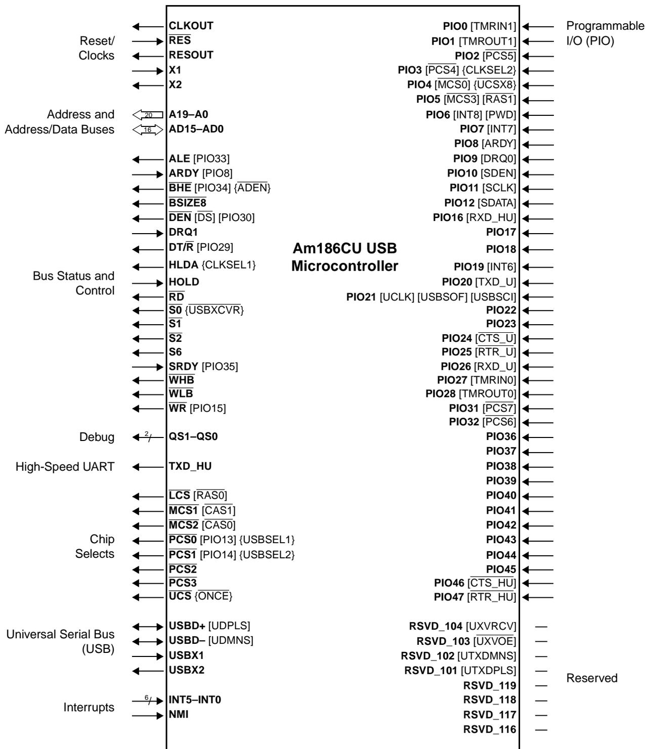
1. Pin names in **bold** indicate the default pin function. Brackets, [ ], indicate alternate, multiplexed functions. Braces, { }, indicate pinstrap pins.
