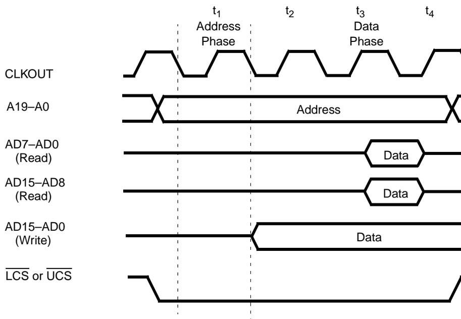
**Figure 4. Am186CU Microcontroller—Address Bus Disable In Effect**
