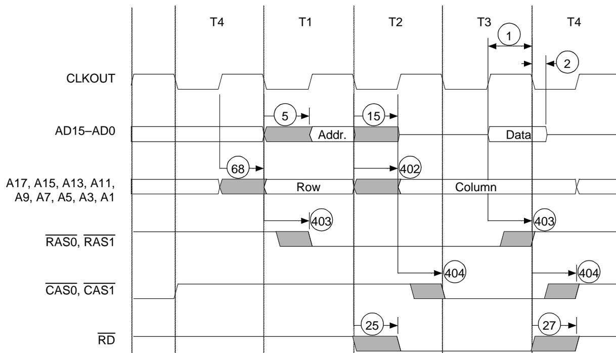
**Figure 30. DRAM Read Cycle without Wait States Waveform**
