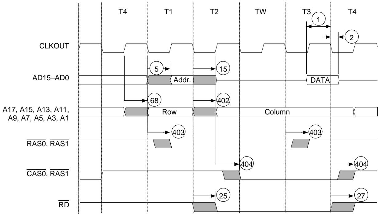
Figure 31. DRAM Read Cycle with Wait States Waveform
