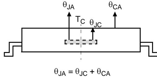
**Figure 11. Thermal Resistance(°C/Watt)**
