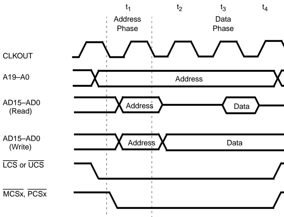
**Figure 3. Am186CU Microcontroller Address Bus — Default Operation**
