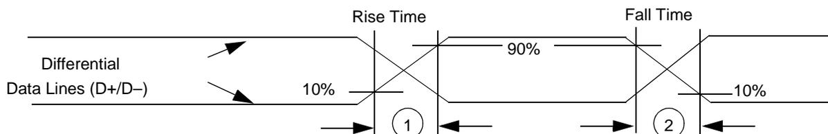
Figure 27. USB Data Signal Rise and Fall Times
