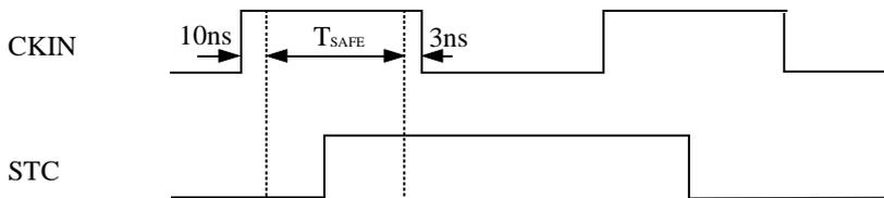
The A/D Converter operates data conversion when STC (Start Conversion) signal is just "HIGH". Otherwise, output data (DO[11:0]) keep the current states. The STC signal should be changed during "T<sub>SAFE</sub>" with the "HIGH" level of the clock to operation as shown in the main waveform.
