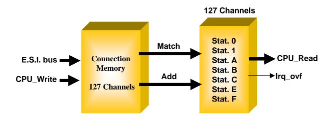
The MESC\_PM1 Controller is composed of two main functions.
