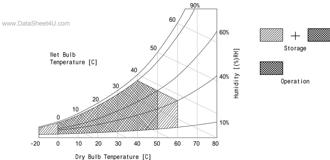
Figure 2. Temperature and relative humidity
