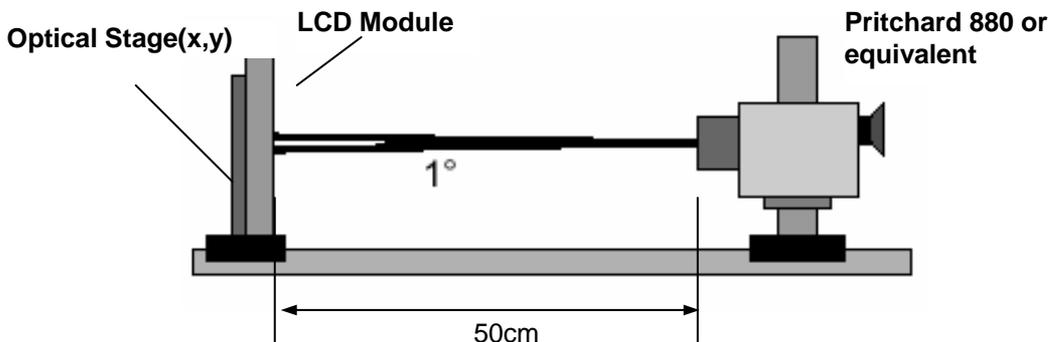
[Figure 5] Optical characteristic measurement equipment and method
