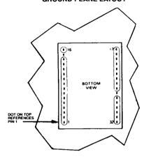
Figure 3. Ground Plane Layout
