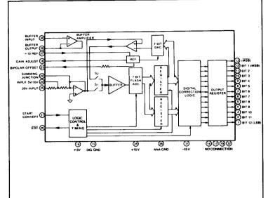
Figure 1. ADC-817A,-827A Simplified Block Diagram
