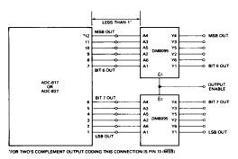
Figure 4. High Speed Three-State Output Buffer
