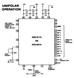
\*FOR GREATER UNIPOLAR ZERO GAIN ADJUSTMENT THE 2 MEG OHM RESISTOR MAY BE REDUCED TO A VALUE OF 500  $\mbox{K}\Omega$
