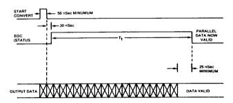
Figure 2. Timing Diagram for ADC-817A, ADC-827A
