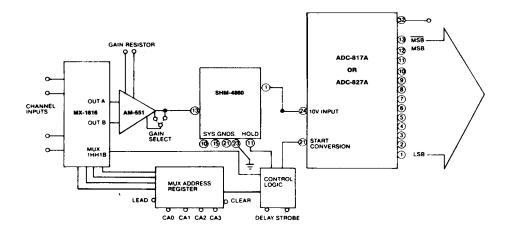
Figure 5. High Speed Data Acquisition System
