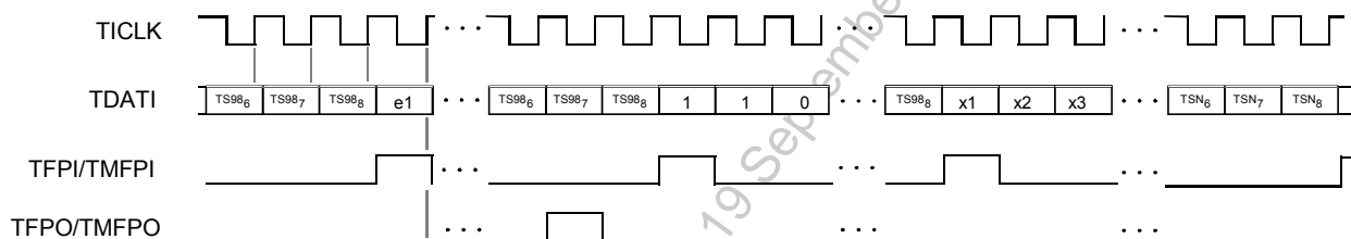
Figure 69 Framer Mode J2 Transmit Input Stream
