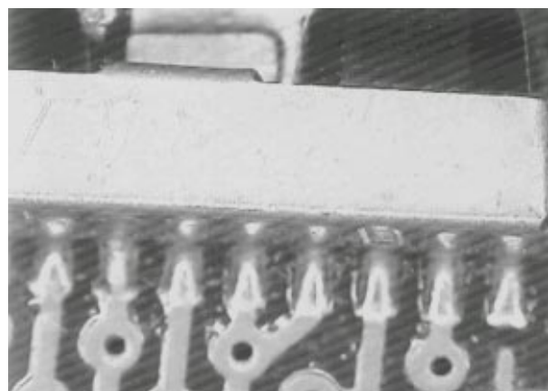
Photo 4.0. Unit self-aligns after reflow.
