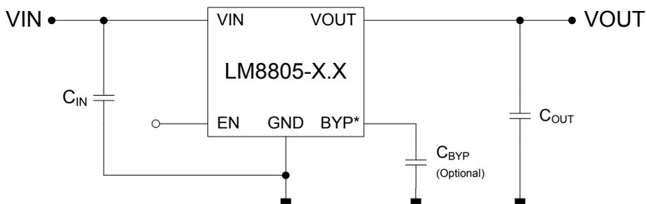
\* Note) BYP pin can be left open if low noise operation is not required.
