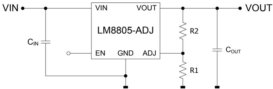
$$V_{OUT} = V_{ADJ}(1+R2/R1)$$
