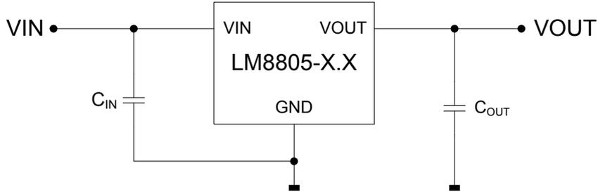
Typical 5 Pin Application Circuit
