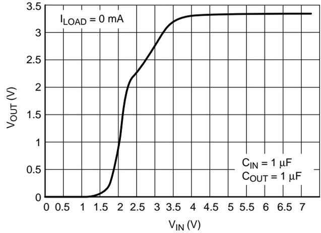
Figure 11.  $V_{OUT}$  vs.  $V_{IN}$  ( $V_{OUT} = 3.3\text{ V}$ )
