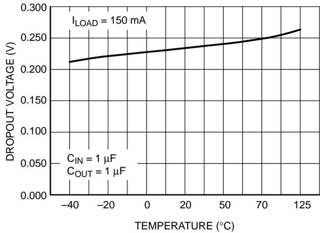
Figure 7. Dropout Voltage vs. Temperature ( $V_{OUT} = 3.3\text{ V}$ )
