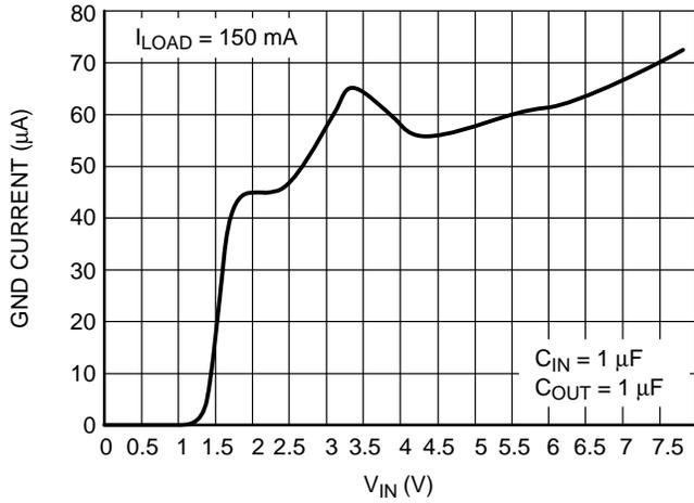
Figure 10. Ground Current vs.  $V_{IN}$  ( $V_{OUT} = 3.3\text{ V}$ )
