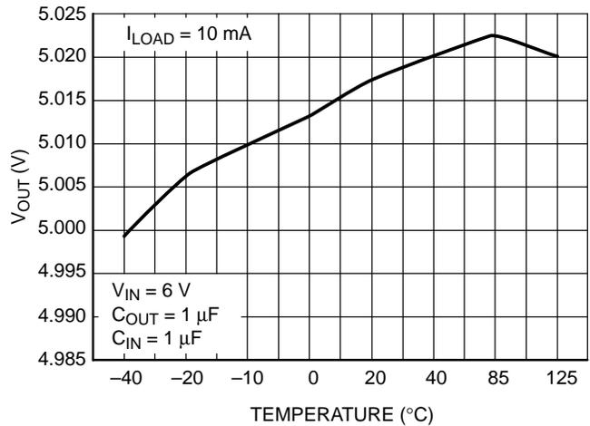
Figure 15. Output Voltage vs. Temperature ( $V_{OUT} = 5\text{ V}$ )
