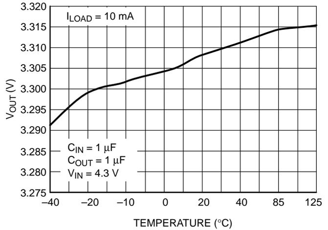
Figure 13. Output Voltage vs. Temperature ( $V_{OUT} = 3.3\text{ V}$ )
