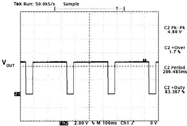
$I_{LOAD}$  was increased until temperature of die reached about 160°C, at which time integrated thermal protection circuitry shuts the regulator off when die temperature exceeds approximately 160°C. The regulator remains off until die temperature drops to approximately 150°C.
