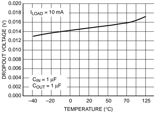
Figure 4. Dropout Voltage vs. Temperature ( $V_{OUT} = 3.3\text{ V}$ )
