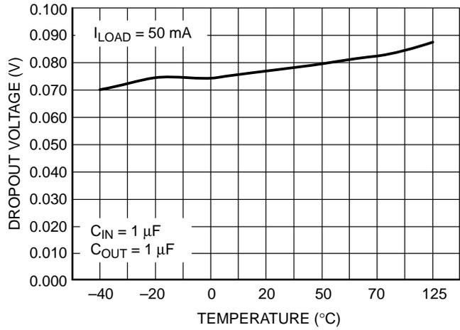
Figure 5. Dropout Voltage vs. Temperature ( $V_{OUT} = 3.3\text{ V}$ )
