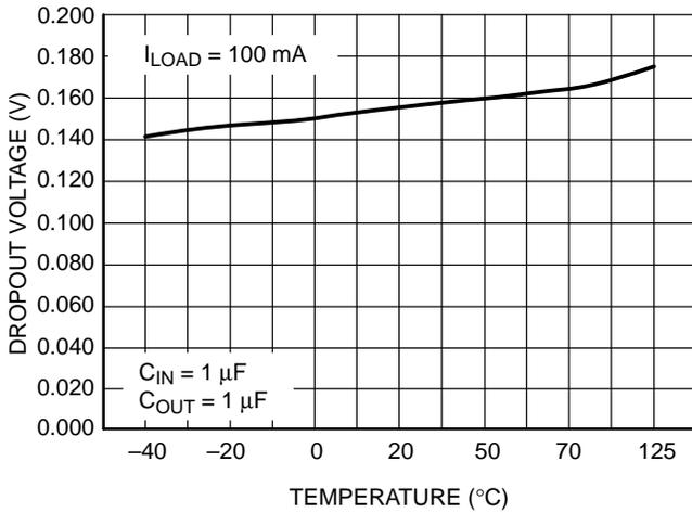
Figure 6. Dropout Voltage vs. Temperature ( $V_{OUT} = 3.3\text{ V}$ )
