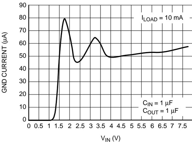
Figure 8. Ground Current vs.  $V_{IN}$  ( $V_{OUT} = 3.3\text{ V}$ )
