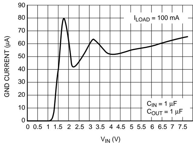
Figure 9. Ground Current vs.  $V_{IN}$  ( $V_{OUT} = 3.3\text{ V}$ )
