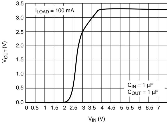
Figure 12.  $V_{OUT}$  vs.  $V_{IN}$  ( $V_{OUT} = 3.3\text{ V}$ )
