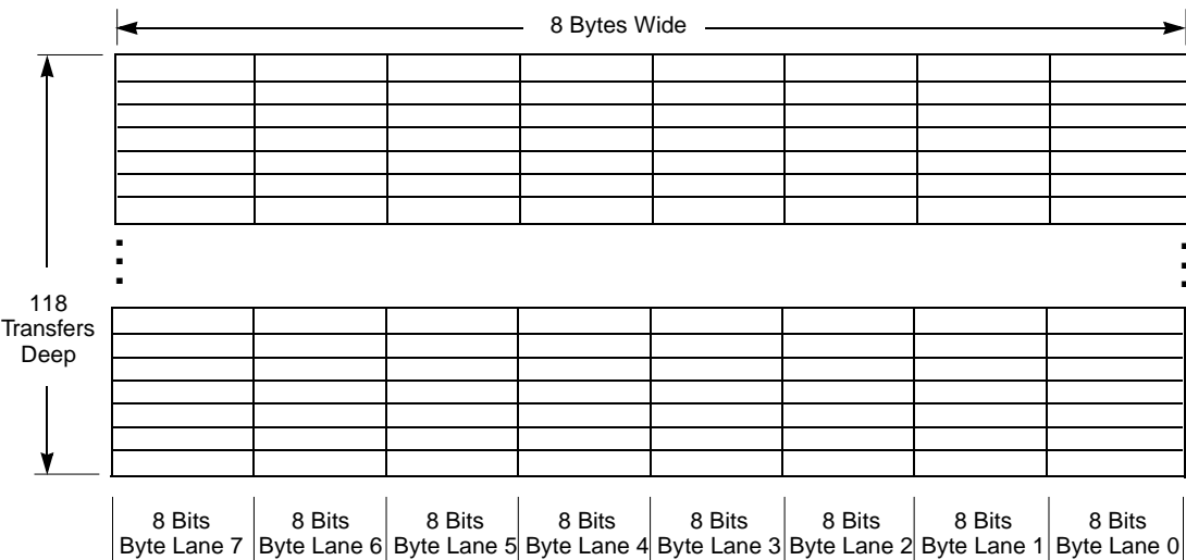
Figure 2.3 DMA FIFO Sections
