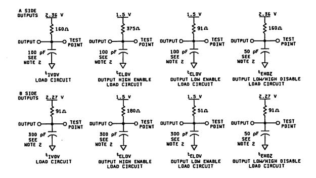
Note:  $V_{IL}$  = 0.4 V,  $V_{IH}$  = 2.6 V except for pin 11 ( $V_{CC}$  - 0.5 V). Includes jig and stray capacitance.
