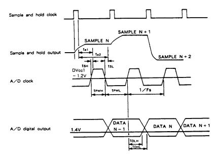
Th is the timing of latching result for the comparation of Vin and Vier the upper comparators. This the timing of latching result for the comparation of Vin and Vier in the lower comparators.
