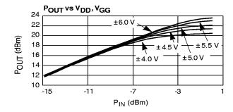
1. Unless otherwise noted, Frequency: 2.45 GHz,  $V_{DD}$  = 5 V ±5%,  $V_{GG}$  = - 5 V ±5%,  $T_{A}$ = +25°C
