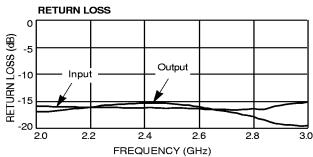
1. Unless otherwise noted, Frequency: 2.45 GHz,  $V_{DD}$  = 5 V ±5%,  $V_{GG}$  = - 5 V ±5%,  $T_{A}$ = +25°C
