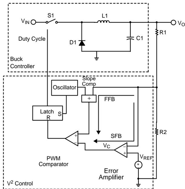
Figure 3. Buck Converter with V<sup>2</sup> Control.
