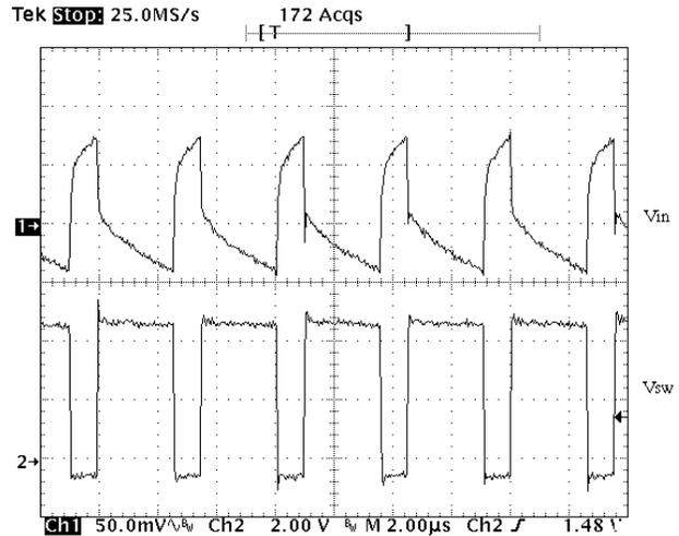
**Figure 11. Input Voltage Ripple in a Buck Converter**
