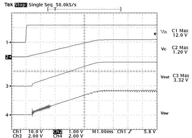
**Figure 8. The Power Up Transition of CS5141X Regulator**
