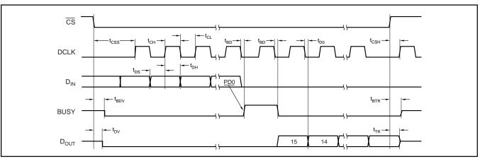
FIGURE 4. Detailed Timing Diagram.
