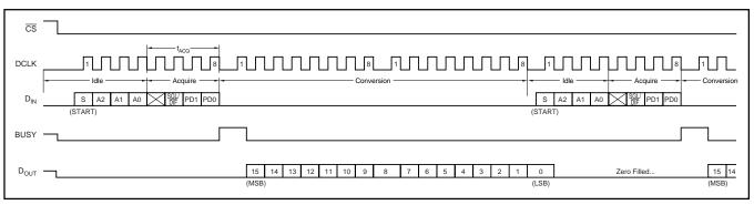
FIGURE 3. Conversion Timing, 24-Clocks per Conversion, 8-Bit Bus Interface. No DCLK delay required with dedicated serial port.
