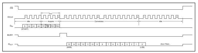
FIGURE 5. External Clock Mode, 32 Clocks Per Conversion.
