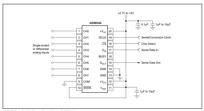
FIGURE 1. Basic Operation of the ADS8344.
