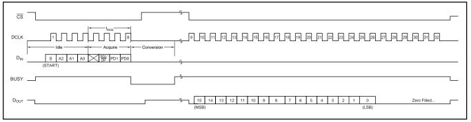
FIGURE 6. Internal Clock Mode Timing.
