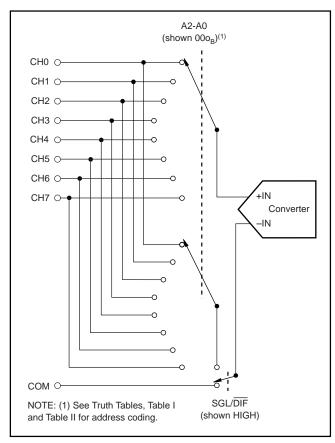
FIGURE 2. Simplified Diagram of the Analog Input.
