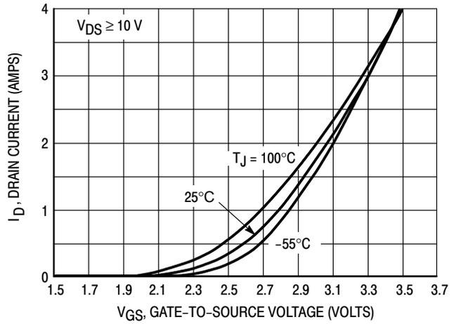
Figure 2. Transfer Characteristics
