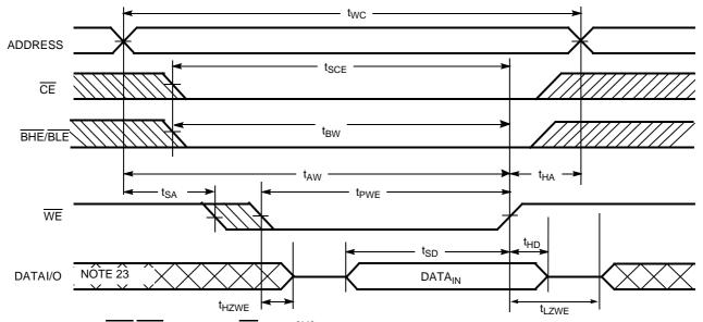
Write Cycle No. 4 (BHE/BLE Controlled, OE LOW)<sup>[22]</sup>
