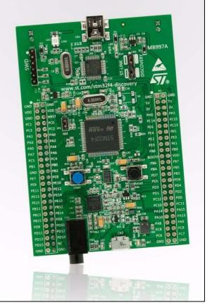
Based on the STM32F407VGT6, it includes an ST-LINK/V2 embedded debug tool, two ST MEMS, digital accelerometer and digital microphone, one audio DAC with integrated class D speaker driver, LEDs and push buttons and an USB OTG micro-AB connector.
